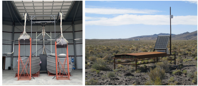
FIG. 3. Left: Photograph of TALE telescopes at the FD station. Right: A deployed SD in the experimental site.
