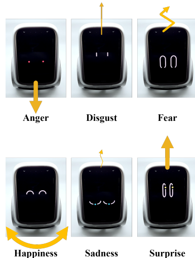
Fig. 1. Emotional expression of the prototype robot. The yellow arrows visualize the movement patterns for six emotions, with thickness indicating speed.
