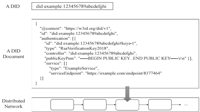
Fig. 9. The examples of a DID and its DID document are shown. The DID consists of a URL scheme identifier, the name of the DID method, and the method-specific identifier. The DID is used to fetch its DID document that has information about the DID subject, such as its public key and service point.
