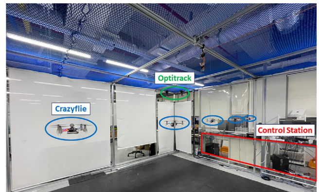
FIGURE 7 Indoor testing environment ( 6 \text{ m} \times 6 \text{ m} horizontal space) for rigid shape formation flight with five Crazyflie quadrotors and a motion tracking system. To ensure formation, quadrotors are set to maintain an equal distance between neighbouring while aligning in a circular pattern (radius of 0.5 \text{ m} ).
