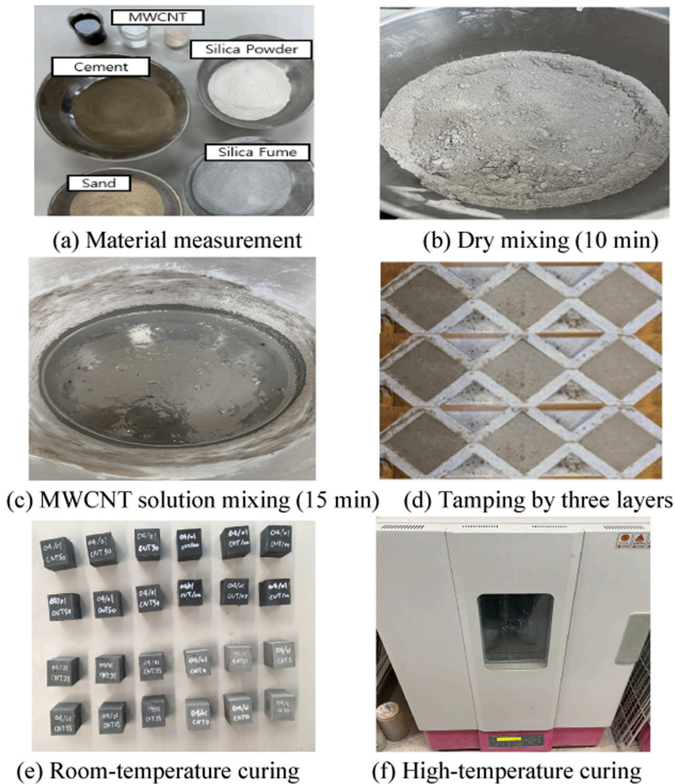
Fig. 1. Multiwalled carbon nanotube ultra-high-performance concrete (MWCNT UHPC) composite fabrication process.
