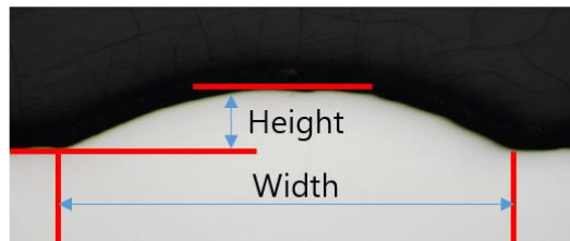
Figure 2.10 Actual deposited (a)dimension and (b)cross-section of single track
