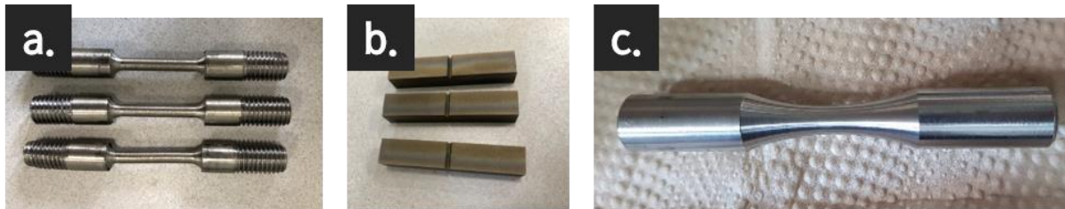
Figure 2.17 (a)Tensile, (b)Impact, (c)Fatigue specimens of optimal parameter
