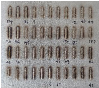
Figure 2.10 Actual deposited (a)dimension and (b)cross-section of single track
