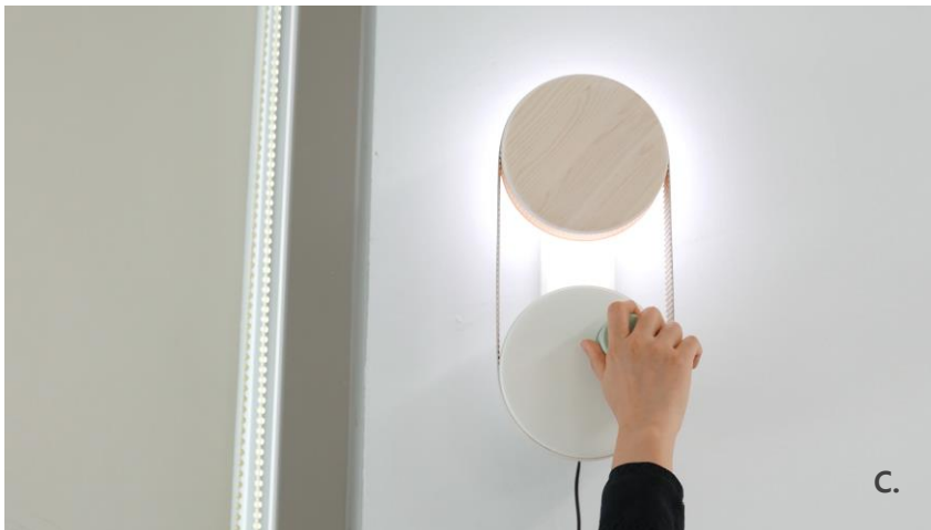
Figure 34 Usage steps of ReeLit. A) take out the button to write goal, B) write what you want to set inside the button, C) Rotating belt and gradual change of light until D-day.
