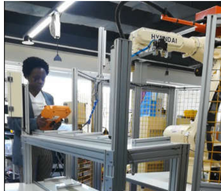
Figure 1.1 Online programming using teach pendant
