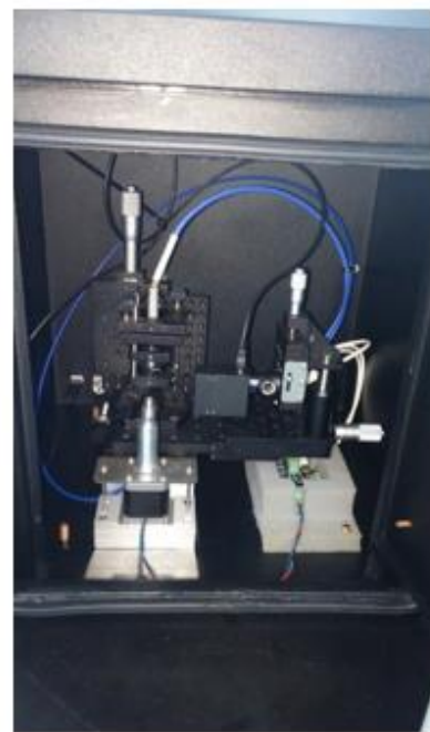
Figure 4.8. (A) Image of disc analyzer for absorbance and chemiluminescence detection. (B) Light blocking black box for containing disc analyzer.
