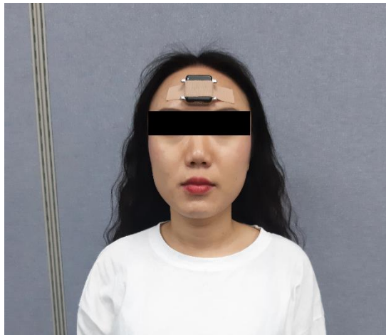
Figure 6. Sensor attachment on participant's middle of forehead
