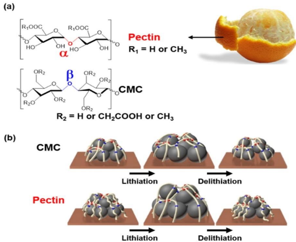
Figure 3. Polysaccharides polymeric binders characterized by glycosidic linkages between their monomeric units and functional moieties on side chains. (a) Molecular structures of polysaccharides: CMC, pectin. (b) Schematic figure of morphological changes of two polysaccharides binders and silicon particles along lithiation and delithiation: white strands = polymeric binders; red points = covalent bonds between hydroxyl and carboxylate moieties of binder; blue points = condensation reaction of between carboxylate of binders and hydroxyl moieties of silicon oxide films on the silicon particles. 3
