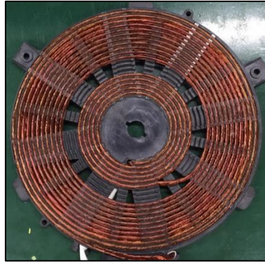
Fig. 14. IH working coil with 16 turns
