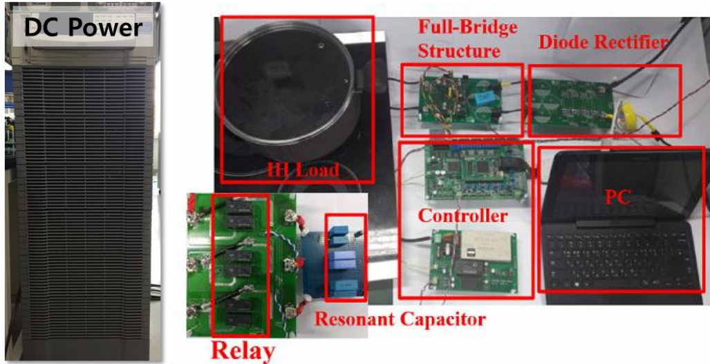
Fig. 37. Experimental setup of 2 kW prototype THM IH system
