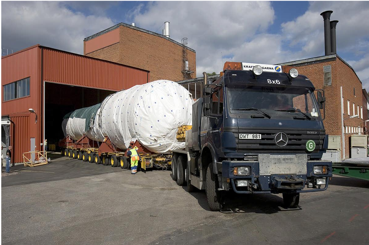
Figure 44. Steam generator transfer
