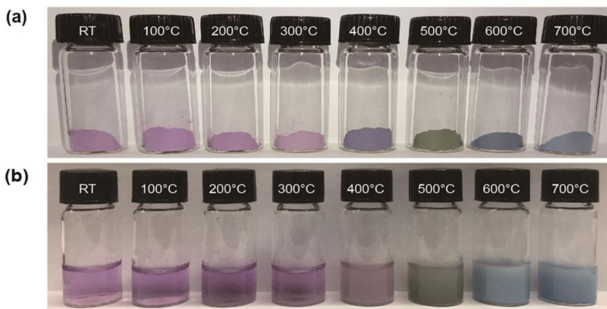
Figure 13. Structural change of POMs by annealing. (a, b) Photographs showing changes in (a) the color and (b) solubility of POMs upon annealing at various temperatures.
