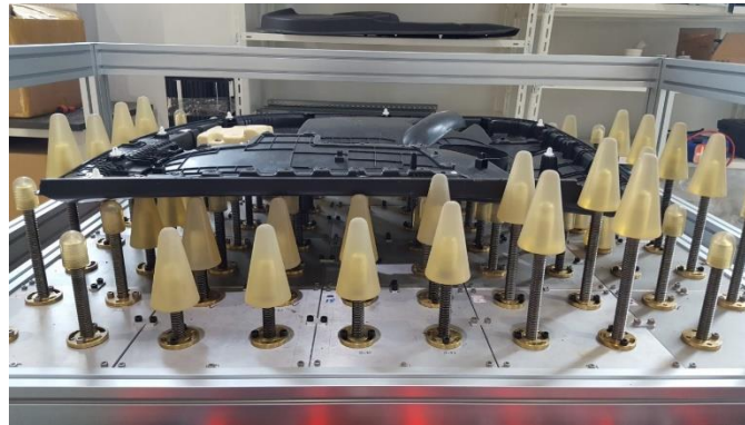
Figure 1-6. Car doortrim panel on the transformable pin-jigs
