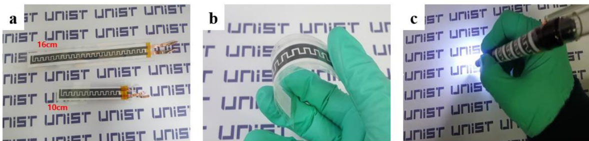
Figure 2.11. Photograph of PAS device depict (a) different size of devices. (b) showing the flexibility of PAS device. (c) operating LED ballpoint pen by PAS in series.
