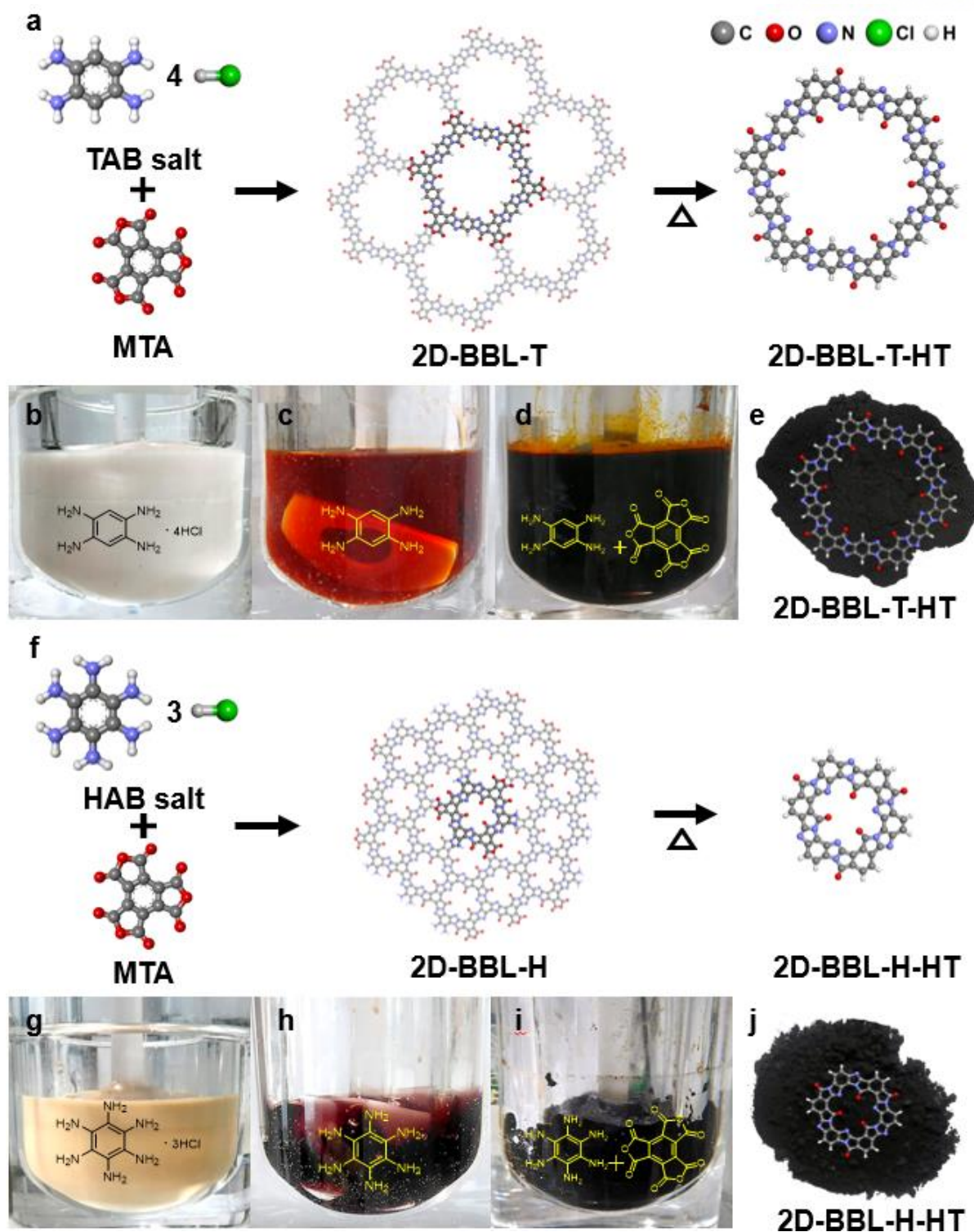
Figure 1.4. (a) Schematic presentation for the formation of 2D-BBL from 1,2,4,5-tetraaminobenzene (TAB) and mellitic anhydride (MA) in polyphosphoric acid (PPA). (b-e) Digital photographs taken during the synthesis of 2D-BBL-T-HT: (b) Tetraaminobenzene (TAB) tetrahydrochloride in PPA at room temperature, (c) after complete dehydrochlorination, the color of media changed from white to orange and transparent. (d) Polymerization with mellitic trianhydride (MTA) at 175 °C. (e) Photograph of as-synthesized 2D-BBL-T-HT. (f) Schematic presentation for the formation of 2D-BBL-H-HT from
