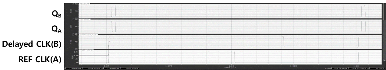
Fig 29. The simulation result of DLL locking between reference clock and delayed clock by controlling CP switches with PFD signal, Q A and Q B
