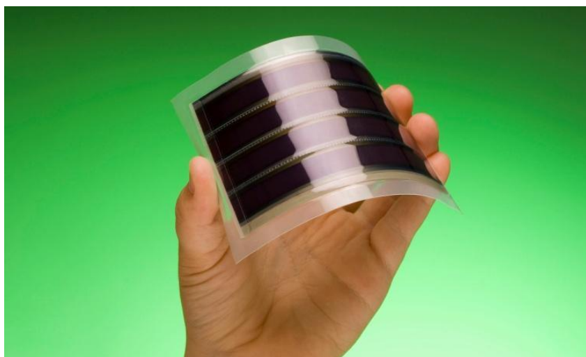
<Figure 11> A flexible dye-sensitized solar cell based on an ITO-PEN substrate.
