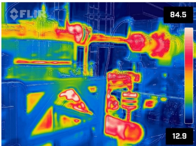
Fig. 18. IR image of the DISNY PRS at P = 155 bar, T = 150 °C operating condition.
