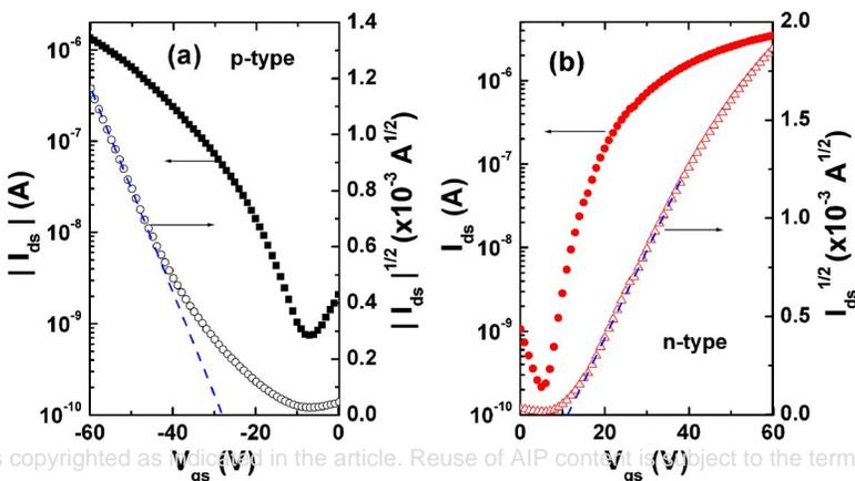
FIG. 3. (Color online) Transfer characteristics of the most optimized bilayer FETs. (a)  $p$ -type operation and (b)  $n$ -type operation. The mobilities deduced from the linear plot of  $I_{ds}^{1/2}$  (the curve plotted by open symbol) were estimated to be  $\mu_e = 8.9 \times 10^{-3} \text{ cm}^2 \text{ V}^{-1} \text{ s}^{-1}$  in the  $n$ -channel mode and  $\mu_h = 5.7 \times 10^{-3} \text{ cm}^2 \text{ V}^{-1} \text{ s}^{-1}$  in the  $p$ -channel mode.
