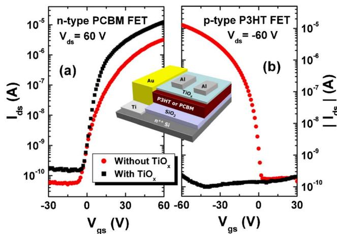
FIG. 2. (Color online) Transfer characteristics of unipolar FETs including a  $\text{TiO}_x$  layer between the active layer and the source-drain electrodes. (a)  $n$ -type PCBM FET and (b)  $p$ -type rr-P3HT FET. For both cases, the data plotted by filled circle (red) represents the devices without  $\text{TiO}_x$  and the data of filled rectangular (black) is for the devices with the  $\text{TiO}_x$  layer.
