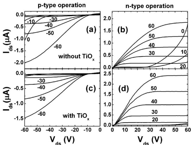
FIG. 4. Output characteristics ( $I_{ds}$ - $V_{ds}$  plots) of the bilayer devices with and without the  $\text{TiO}_x$  separating layer. The data in (a) and (b) were obtained from bilayer FETs without the  $\text{TiO}_x$  separation layer (fabricated by thermal evaporation of  $\text{C}_{60}$ ). The data in (c) and (d) were obtained with the  $\text{TiO}_x$  separating layer (see Fig. 1).
