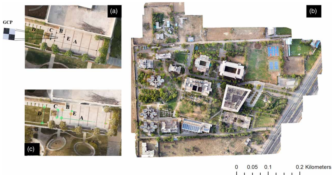
Figure 5 | Images of (a) selected features for physical measurement; (b) digital orthomosaic of the mapped area; and (c) digital measurements of the selected features on the developed orthomosaic.
