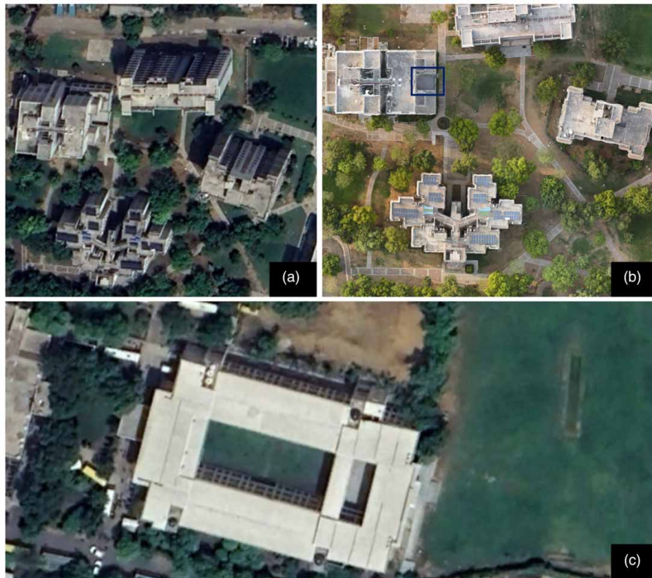
Figure 2 | Satellite imagery showing (a) tilted view of buildings in satellite imagery; (b) features that are not a part of building roof; and (c) appearance of corrugated metal roof in satellite imagery.
