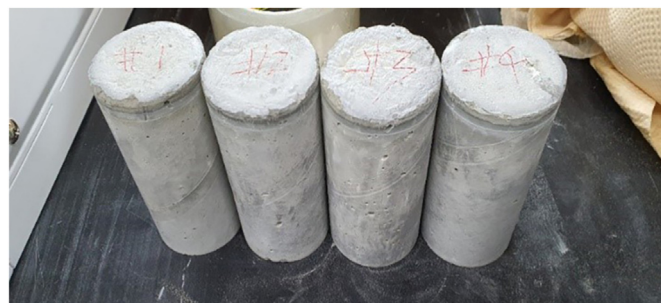
Fig. 1. Waste samples produced with cement solidification.
