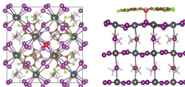
**Fig. 1** Optimized structure of  $F_{16}\text{ZnPc}$  adsorbed on  $\text{MAPbI}_3(001)$ , (left) top and (right) side views along [100]. The solid square in the top view denotes a  $2 \times 2$  supercell of a tetragonal primitive cell. Atomic colour scheme: Pb (grey), I (purple), N (light blue), C (brown), H (white), Zn (red) and F (green).
