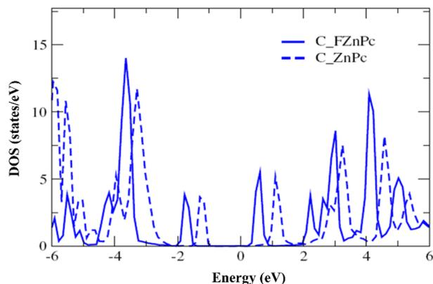
Fig. 3 Comparison of the molecular C PDOS for  $F_{16}ZnPc/MAPbI_3(001)$  (solid line,  $C_{FZnPc}$ ) and  $ZnPc/MAPbI_3(001)$  (dashed line,  $C_{ZnPc}$ ) by adjusting the two vacuum levels to be equal to each other. The positive and negative energy values indicate the unoccupied and occupied states, respectively.
