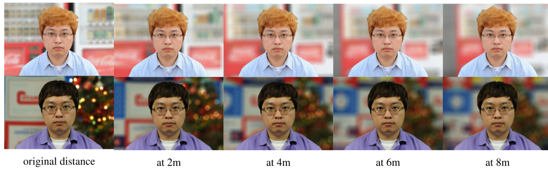
FIGURE 18 Examples of virtual composition at different distances between the camera and the background and the images captured at different distances between the camera and background are shown
