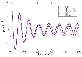
FIG. 8. The Fourier transform coefficient,  $\rho_k(t)$ , for the node number n = 1 is displayed as a function of time. LHV and SMF results are compared to DFS calculations with and without relativistic kinematics.
