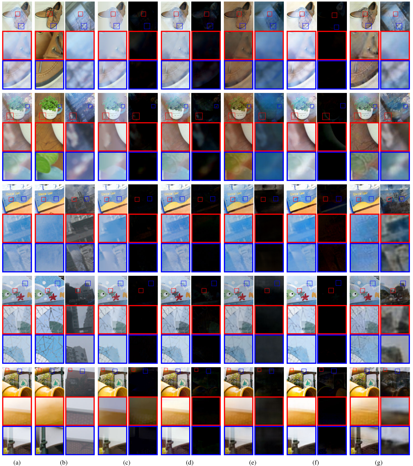
FIGURE 13. Qualitative comparison on our test set. (a) Input glass images. (b) The ground truth transmission (left) and reflection (right) images. The pairs of a transmission image (left) and a reflection image (right) restored by using (c) DFR [14], (d) CEILNet [16], (e) PRRNet [18], (f) BDNet [19], and (g) the proposed network.
