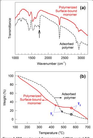
**Figure 3 FTIR spectra and thermograms of PTHA-coated TiO<sub>2</sub> electrodes.** (a) FTIR spectra and (b) thermograms of PTHA-coated TiO<sub>2</sub> electrodes for surface-bound polymerization versus direct polymer adsorption. An inert atmosphere was kept at 20°C min<sup>-1</sup> for TGA.
