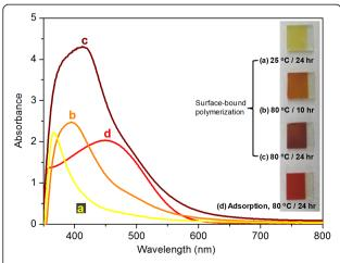
**Figure 2 UV-vis spectra of PTHA-coated TiO<sub>2</sub> electrodes.** (**a**, **b**, **c**) PTHA prepared by surface-bound polymerization with various oxidizing conditions: dipping in FeCl<sub>3</sub> (a) at room temperature for 24 h, (b) at 80°C for 10 h and (c) at 80°C for 24 h. (**d**) PTHA prepared via direct polymer adsorption by dipping TiO<sub>2</sub> electrodes in PTHA solution at 80°C for 24 h. (Inset) Photograph of PTHA-coated TiO<sub>2</sub> electrodes.
