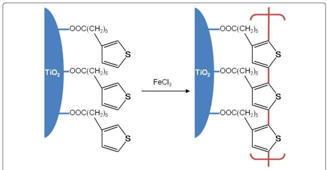
Figure 1 Surface-bound polymerization of THA to PTHA on surface of a TiO<sub>2</sub> nanocrystallite. The monomer THA was strong bonded to TiO<sub>2</sub> surface via -COOH. FeCl<sub>3</sub> was used as an oxidizing agent to polymerize the surface-bound THA to its corresponding polymer PTHA.
