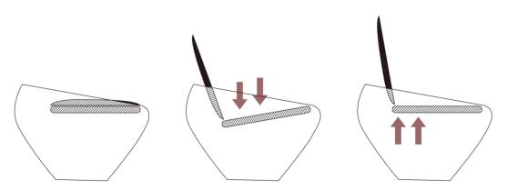
Figure 4. Working process of the seat of the waterless toilet prototype.
