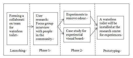
Figure 1. Co-designing a waterless toilet using the fuzzy front end (FFE) process.
