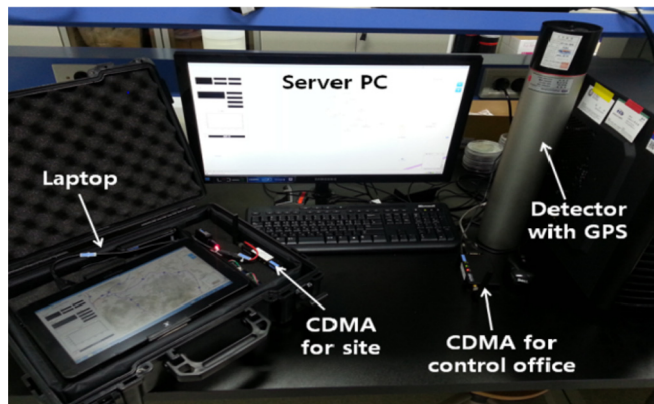
Fig. 4. The system components of the gamma dose rate distribution monitoring system.
