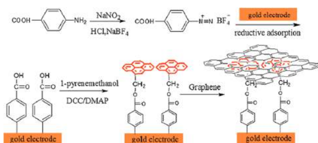
Figure 40. Pyrene interconnection between G and gold electrode. Reprinted with permission from ref 164. Copyright 2013 Elsevier B.V.
