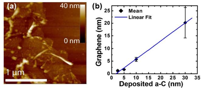
FIG. 4. (Color online) (a) AFM image of a transferred graphene sheet on a Si/SiO<sub>2</sub> substrate. (b) Graphene (and graphite) thickness vs initial a-C thickness. Samples were annealed at 800 °C for 15 min with a 300 nm Ni catalyst layer.
