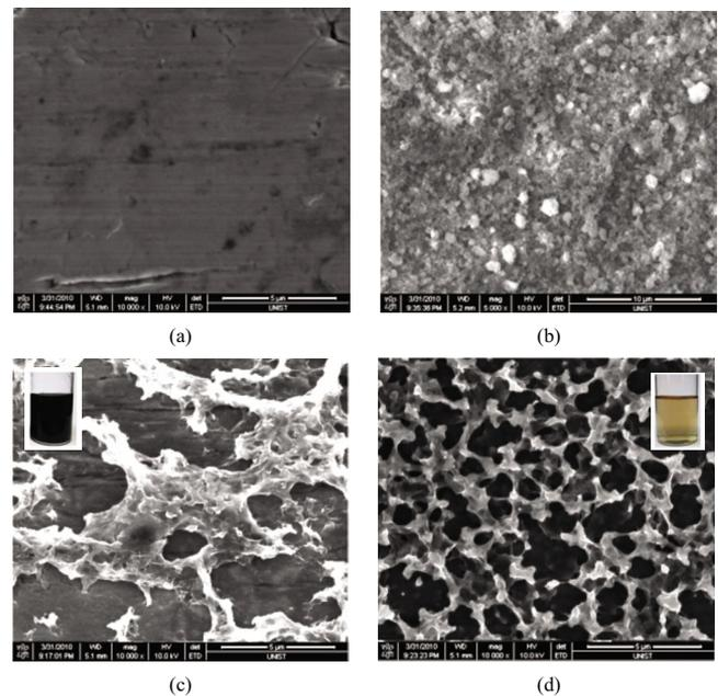
FIG. 1. (Color online) SEM image ( $\times 10\,000$ ) of heater surface after pool boiling in (a) base-fluid water, (b) Al<sub>2</sub>O<sub>3</sub> nanofluid, (c) graphene nanofluids, (d) graphene oxide nanofluid. (Insets in (c) and (d) are graphene and graphene oxide nanofluids, respectively).
