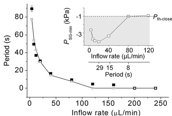
FIG. 4. Effect of  $P_{th-close}$  on the operational range of the inflow rate. Filled and unfilled points are the experimental and simulation results, respectively.  $R_d + R_c$  is  $1.7 \times 10^{13} \text{ N}\cdot\text{s}/\text{m}^5$ . Gray region ( $P_{SG-min} < P_{th-close}$ ) of the inset is oscillation region.
