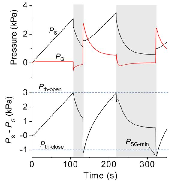
FIG. 2. Simulated source and gate pressure profiles of valve 2 at the onset of oscillation.  $Q_i$  is 2  $\mu\text{l}/\text{min}$ . Gray region corresponds to valve 2-on state. At the bottom panel,  $P_{\text{SG-min}}$  is a minimum value of  $P_S - P_G$ . If  $P_{\text{SG-min}}$  is  $> P_{\text{th-close}}$  at the moment of valve 1-on to valve 2 off, valve 2 stays on. As a result, both valves are on and oscillation stops.
