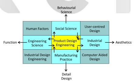
**Figure 1** The influences and connections of product design engineering in a product development context (Adapted from Dixon, 1966, in Hundal 1997, p. 38).
