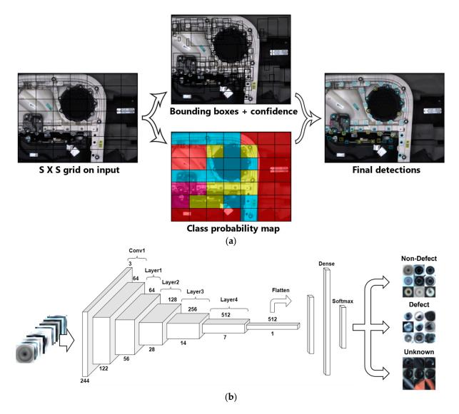
**Figure 1.** (a) YOLO flowchart for detecting quality of heat staking points in door trim images and (b) ResNet flowchart for classifying the quality of heat staking points.
